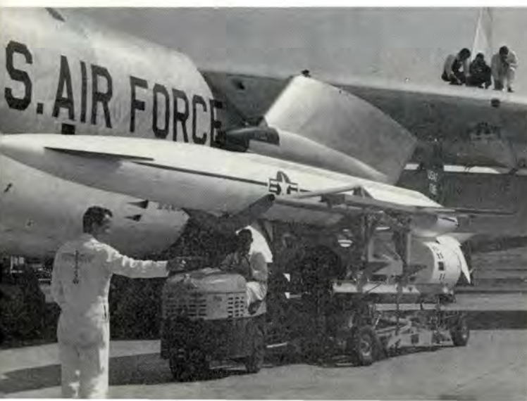
Upper left, flight attitude positioner is rock-and-roll device to simulate flight conditions. Lower left, Air-Log positioning trailer is rolled under wing, preparatory to mating the missile to its carrier. Lower right installation nears completion.
