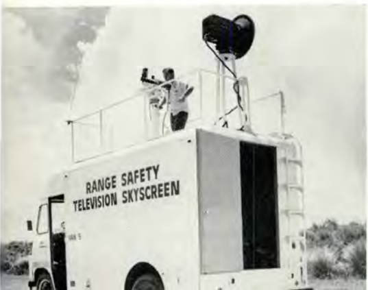
Left, two TV cameras are used for each launching and data sent to Range Safety Console. Right, a simple vertical wire skyscreen allows Range Safety Officer to judge deviation during lift off. Parallel wires are coated with fluorescent material and illuminated by black light for night launching.
