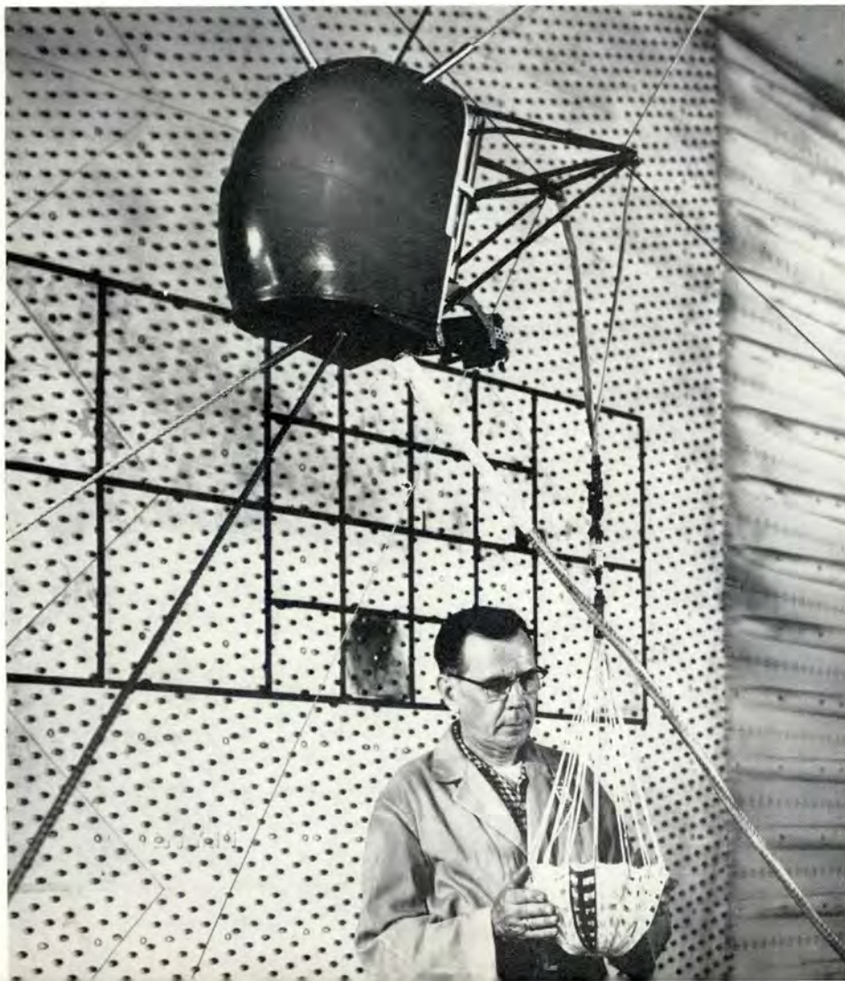
Below left, proposed B-58 escape capsule in 16-ft. transonic wind tunnel. Drogue chute offers maximum drag and stabilization. Right, strip from motion picture footage during test opening at simulated speed of 505 knots.
