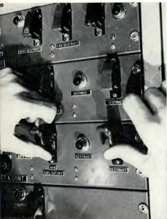
Above, RSO's reaction time to destroy errant missile is 2 sec. Below, high speed digital computer automatically determines point of missile impact should thrust be terminated.
