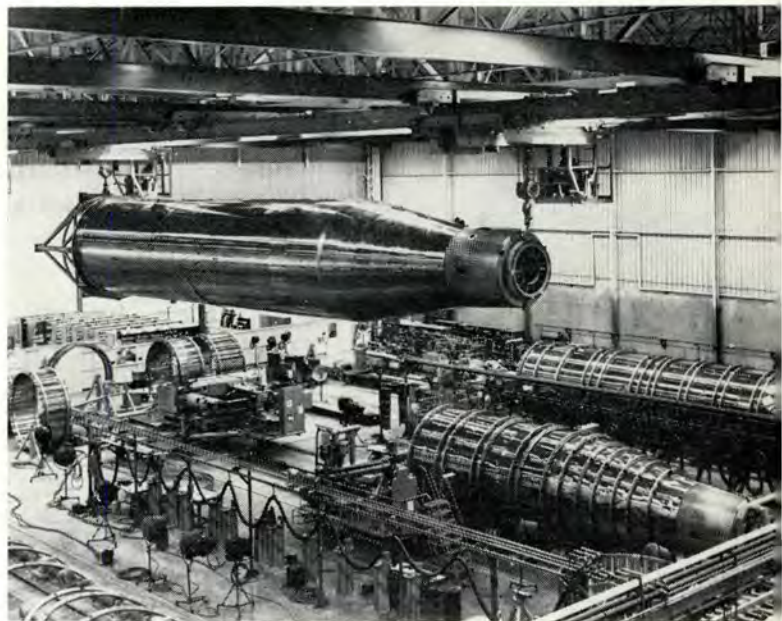
Left, welded bands of thin, stainless steel make up tank sections. Note the near-surgical cleanliness of work area and material. This is imperative for safe missile operation from factory to launch. Right, the 60-ft. tank is completed. It is now pressurized to enable it to hold its shape.
