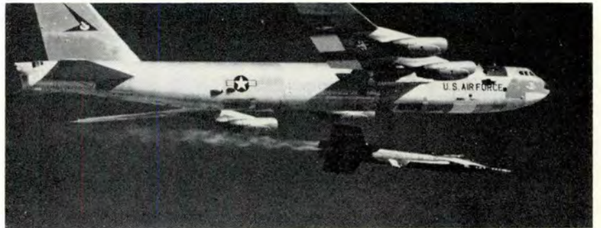
Above, B-52, with X-15 tucked under wing, lifts off. Lower left, specially designed pylon carries the X-15. Lower right, the payoff: with full rocket power, speeds in excess of 3600 mph are expected to be reached.
