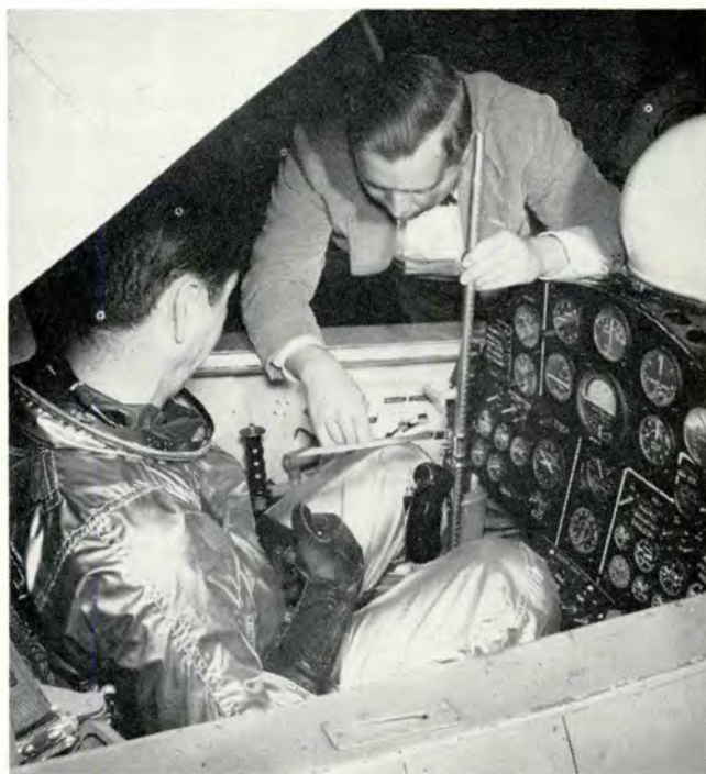
Top left, Scott Crossfield is shown in cockpit prior to a test flight. Lower left, a pilot's eye view of cockpit with canopy in place. Note simplicity of instrumentation. Top right, one of the pilots is measured for adequate cockpit clearance. Each X-15 pilot has an individually tailored seat which, when used with full pressure suit, insures safe ejection at ground level and aerodynamic stability at supersonic airspeed.
