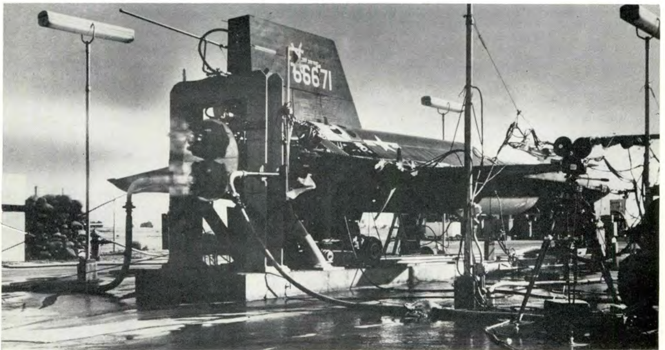
Careful ground checkout of all operating equipment, including engines, precedes each flight of the X-15 from Edwards Air Force Base, Calif.
