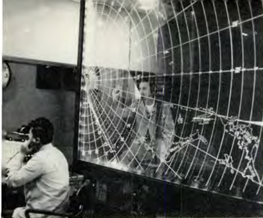
Surveillance Plotting Board shows location of ship and plane in flight path or impact area. Launching of missile is delayed 'til cleared.
