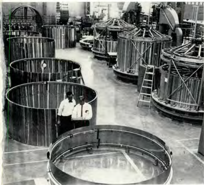
Left, welded bands of thin, stainless steel make up tank sections. Note the near-surgical cleanliness of work area and material. This is imperative for safe missile operation from factory to launch. Right, the 60-ft. tank is completed. It is now pressurized to enable it to hold its shape.
