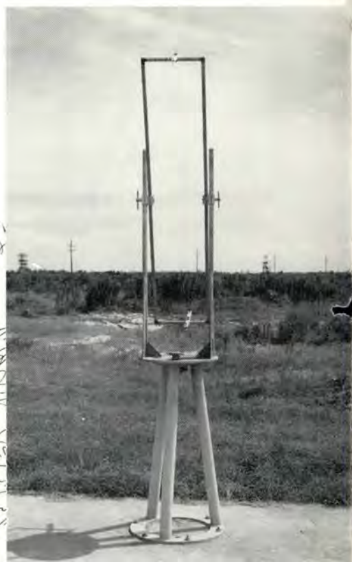
Left, two TV cameras are used for each launching and data sent to Range Safety Console. Right, a simple vertical wire skyscreen allows Range Safety Officer to judge deviation during lift off. Parallel wires are coated with fluorescent material and illuminated by black light for night launching.
