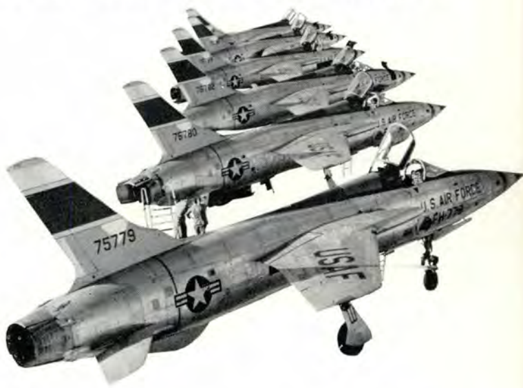
Left, sleek and supersonic, the F-105 presents an imposing appearance. Advance design includes swept-forward air intake ducts. Lower left, unique cloverleaf speed brakes are shown partially open.
