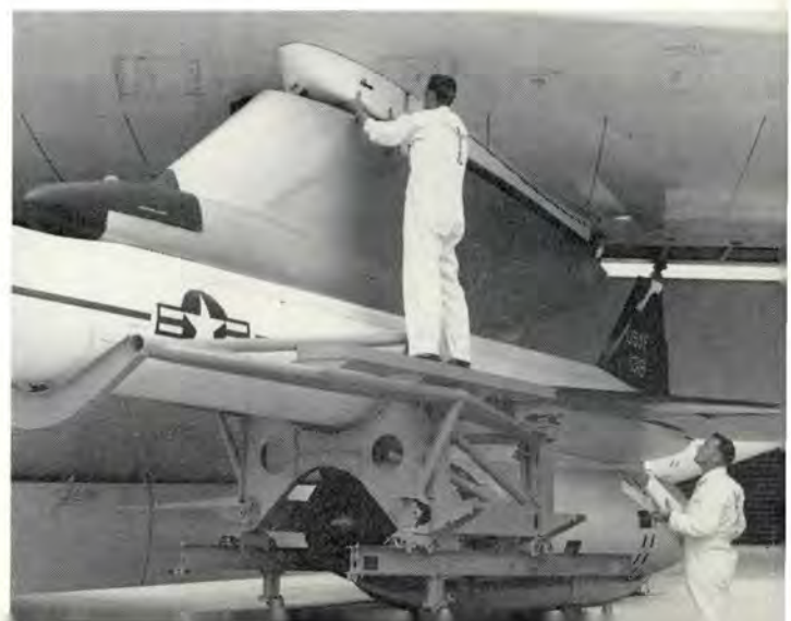
Upper left, flight attitude positioner is rock-and-roll device to simulate flight conditions. Lower left, Air-Log positioning trailer is rolled under wing, preparatory to mating the missile to its carrier. Lower right installation nears completion.
