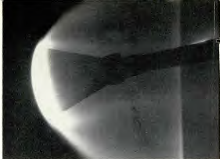
A Mercury man-in-space capsule enveloped in luminescent airflow during Mach 20 test run in Arnold Engineering's tunnel Hotshot Number Two.
