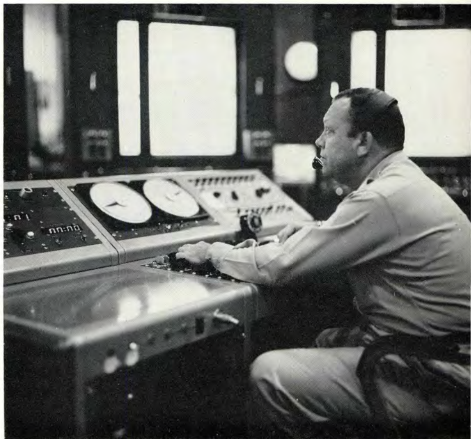
Upper left, optical skyscreen detects deviations from planned trajectory. Upper right, impact predictor plotting board charts missile course and predicts impact point. L/C R. D. Stephens, Senior Range Safety Officer, at console, is responsible for destroying missile headed into danger area.
