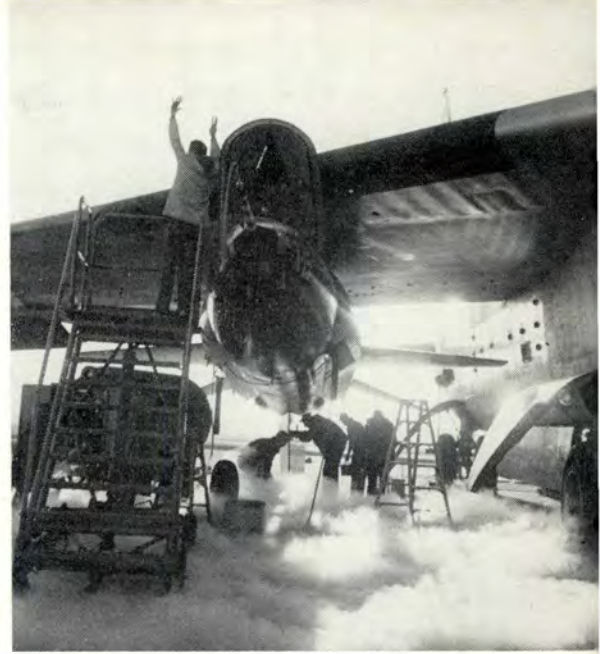
Left, X-15 mated to the B-52. Above, chilled helium is pumped into the X-15 causing ground fog. Chilling the gas makes it possible to increase fuel load.
