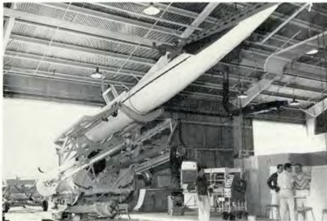
Upper left, flight attitude positioner is rock-and-roll device to simulate flight conditions. Lower left, Air-Log positioning trailer is rolled under wing, preparatory to mating the missile to its carrier. Lower right installation nears completion.
