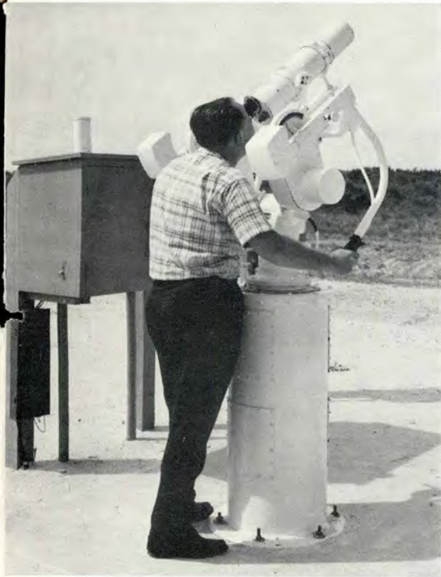
Upper left, optical skyscreen detects deviations from planned trajectory. Upper right, impact predictor plotting board charts missile course and predicts impact point. L/C R. D. Stephens, Senior Range Safety Officer, at console, is responsible for destroying missile headed into danger area.
