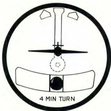
Fig. 1, above, aircraft silhouette attached to TURN NEEDLE; ball is obscured. Fig. 2, right, converted RMI. Fig. 3, below, standard RMI converted to present pitch, roll and heading.
