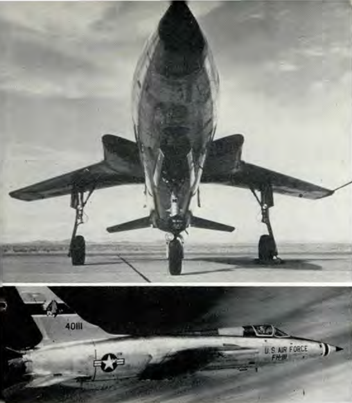
Left, sleek and supersonic, the F-105 presents an imposing appearance. Advance design includes swept-forward air intake ducts. Lower left, unique cloverleaf speed brakes are shown partially open.
