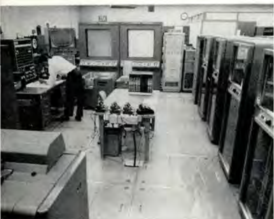
Above, RSO's reaction time to destroy errant missile is 2 sec. Below, high speed digital computer automatically determines point of missile impact should thrust be terminated.
