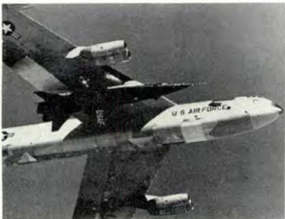
Above, B-52, with X-15 tucked under wing, lifts off. Lower left, specially designed pylon carries the X-15. Lower right, the payoff: with full rocket power, speeds in excess of 3600 mph are expected to be reached.
