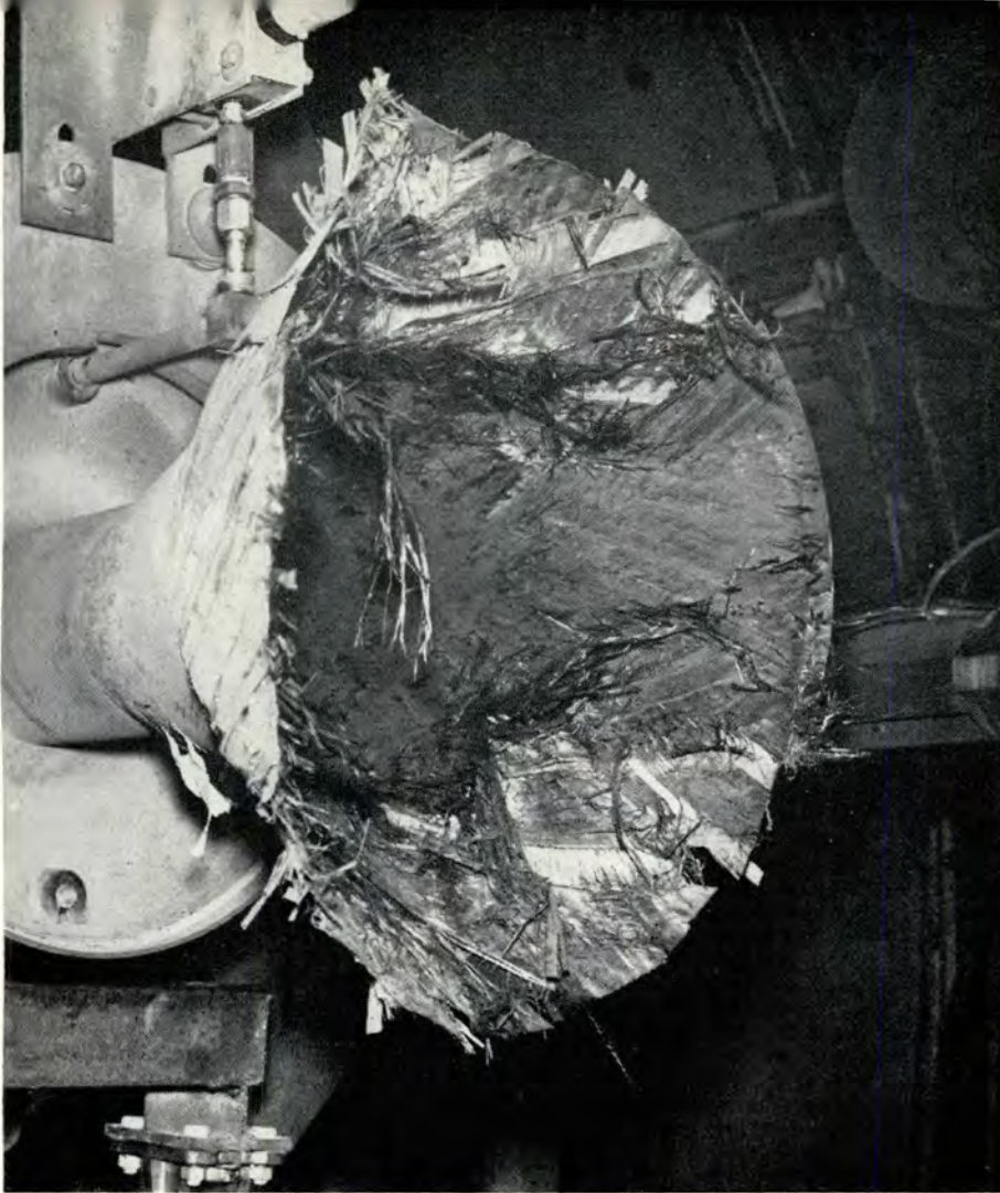
Left, nozzle fails during altitude test. Right series, hot spots start at nozzle exit; burn-through starts at rim; burns off, cone disintegrating.
